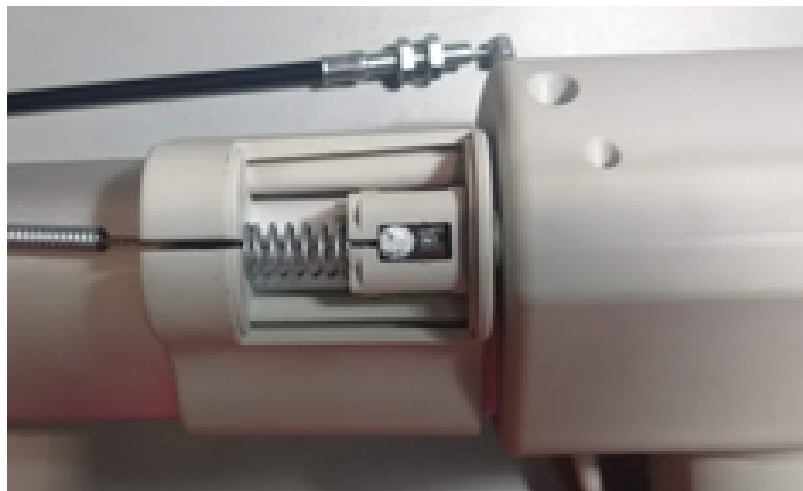
fig 4. Insert AC-32 cable end with spring into housing.
