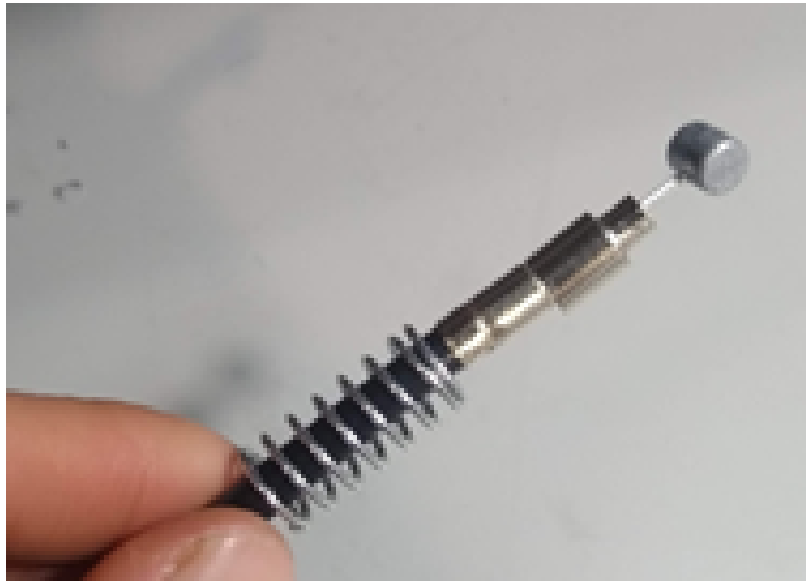
fig 3. Transfer spring from housing to AC-32 cable end.
